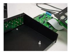
Remount the back board into the mixer case with it's five screws. Plug the main board into the back board with the multi-pin connector and secure the main board onto the bottom of the mixer with its' screws. Make sure you use the stand off spacers to keep the main board fixed in place.
