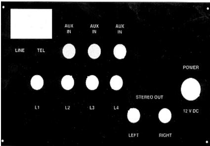
CD/MP3 players in the console and accept audio going to the mixer from 3 RCA jacks and a telephone interconnect jack on the back of the console.
